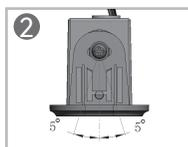
Adjust the sensor's detection angle.
