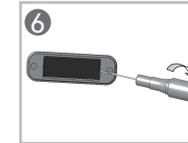
Gently lift the front cover with a screwdriver as shown.
